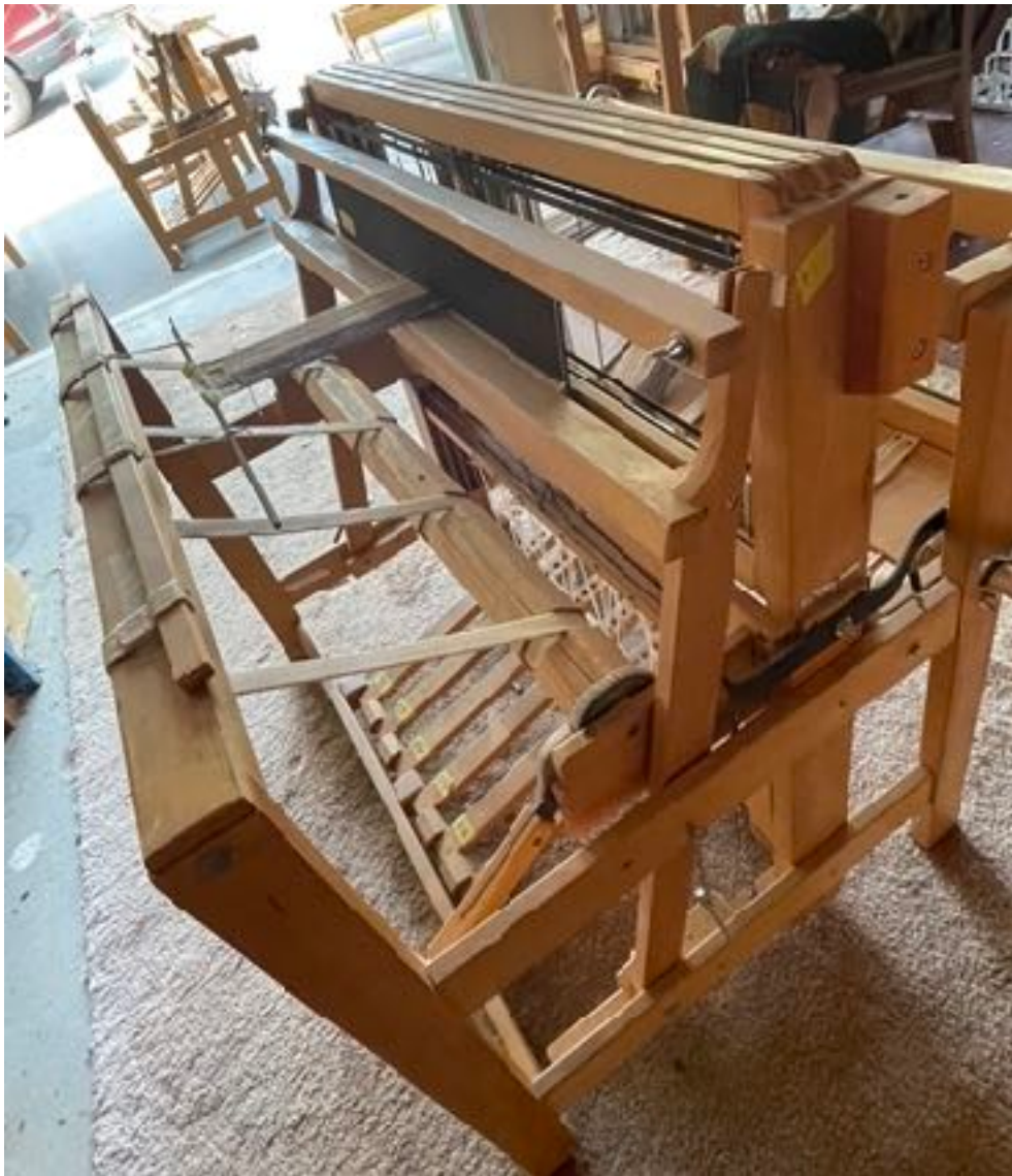
This loom has been altered to have a lease stick holding device built in
